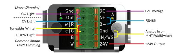
The full PoE Voltage is output at the "DC" terminal. RS485 is available at A+ and B-. An analog sensor or an MHTi Wall Switch can be connected at "IN/WS". And a +24V output is also available to power external sensors.
